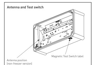
The test switch on this product is a magnetic type so that the weatherproof seal does not have to be opened. To perform a manual test, hold a magnet against the product surface near the "Magnetic Test Switch" label. A magnet is provided with the product. This magnet should not be left attached to the magnetic test switch during installation.
